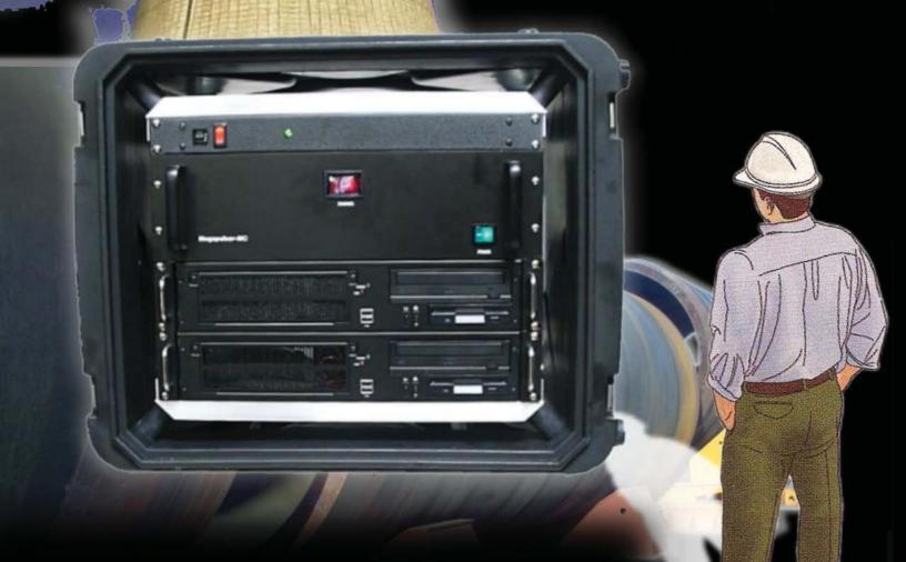
Combination ultrasonic and laser displacement system. When combined with the AIS RoboScanner, this system records high resolution Corrosion mapping fast and efficiently. Use our dual crystal straight beam for far surface mapping (thickness and corrosion measurement). Switch to our high resolution laser displacement sensor to record near surface (OD) corrosion.
