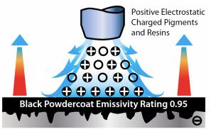
Original Aluminum Part Surface Emissivity Rating 0.07
