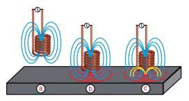
a - The alternating current flowing through the coil at a chosen frequency generates a magnetic field around the coil.
