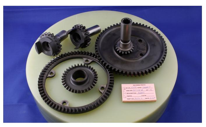
Magneto & Accessory Drive Gear Oil Pump and Tach Shaft Gear Alternator Drive Face Gear
