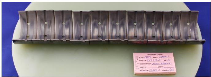
Main Crankshaft Bearing Part # SA-642839
