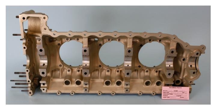
After Black Electrostatic Powder Coating Removed - Crankcase ENGINE S/N 267651-R
