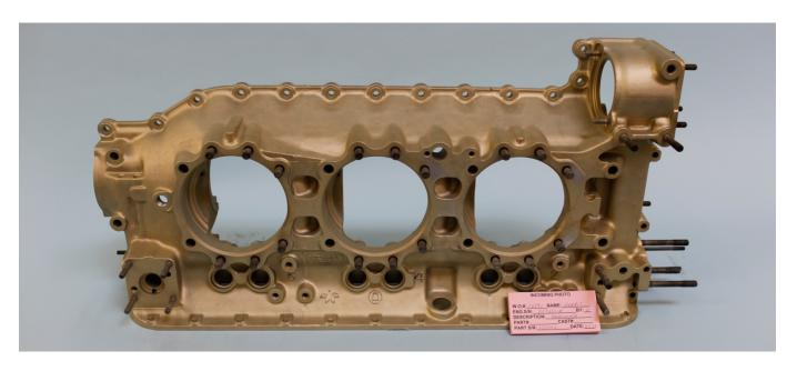
After Black Electrostatic Powder Coating Removed - Crankcase ENGINE S/N 267651-R
