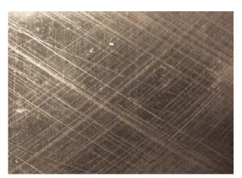
Above - Inside View - Superior Cylinder Barrel Wall Surface Part #SA5H52000-A1 (Magnified View) Cylinder bore surface showing cross-hatch machine marks.
