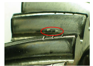
Fig. 10 Pitting condition after testing
