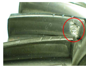
Fig. 10 Pitting condition after testing
