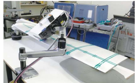
Pulstec X-360n X-Ray Diffraction - 90 degree position. Photo: Victor Aviation Service
