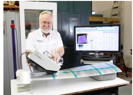
Pulstec X-360n X-Ray Diffraction Testing / NASA Turbine Blade - 0 Degree Position. Photo: Victor Aviation Service
