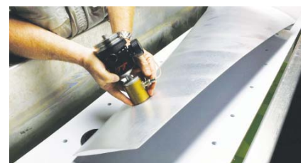
Dual Polarized EMAT Testing / NASA 11-by-11-foot Transonic Unitary Wind Tunnel Turbine Blade. Photo: Victor Aviation Service
